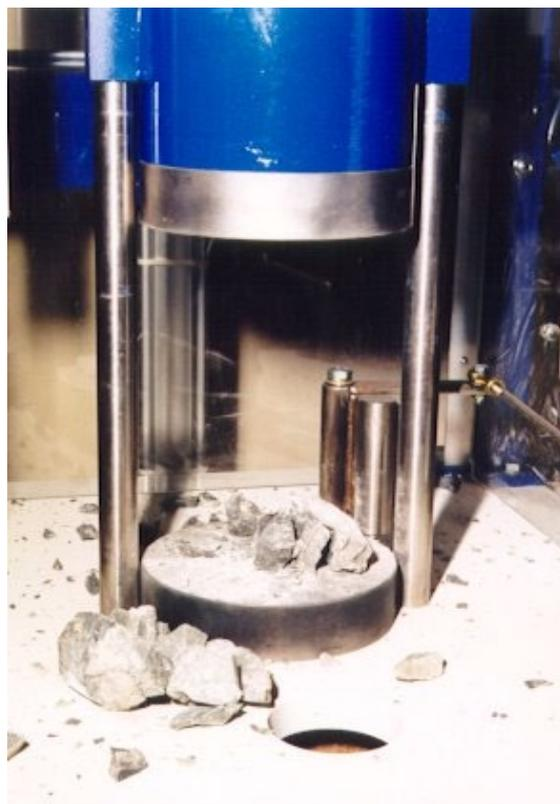
Figure 7 – JK Drop-weight Tester Impact Head and Anvil
