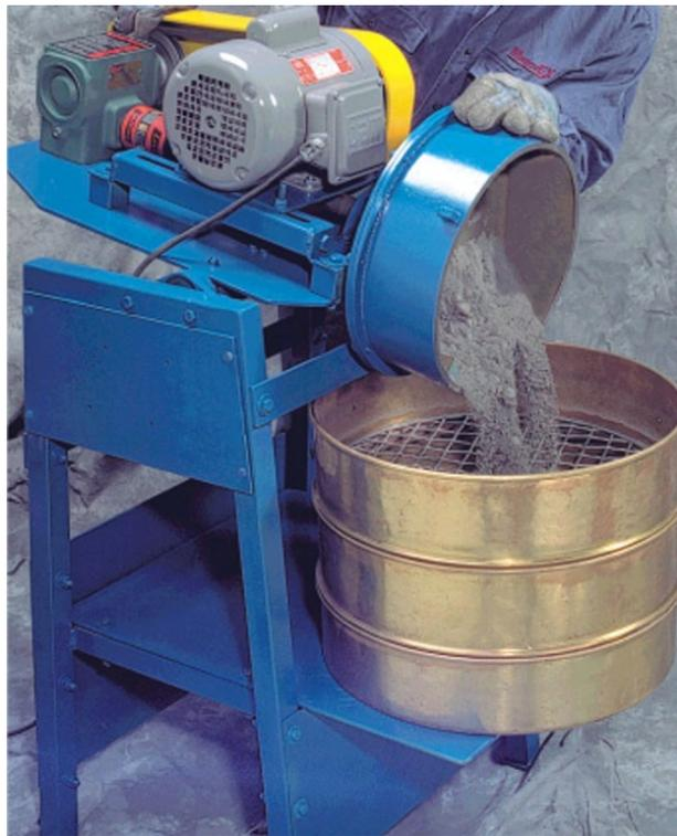
Figure 5 - SPI Laboratory Test Mill (After Amelunxen, 2003)
