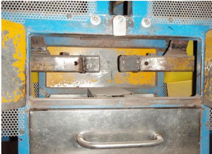
Figure 2 Region where breakage takes place in Bond's crushing work index machine
