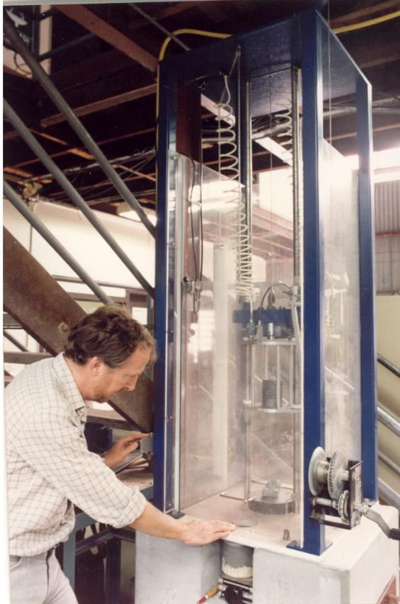
Figure 6 – Original JK Drop-weight Tester
