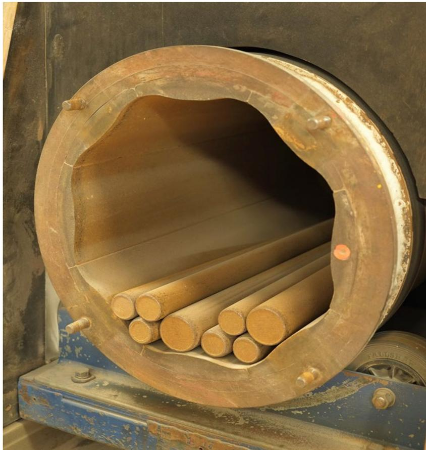
Figure 3 - Bond rod mill
