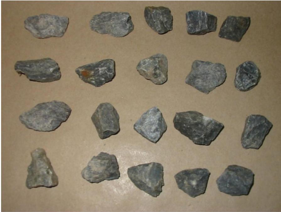
Figure 10 Particles selected for SMC testing from crushed rock
