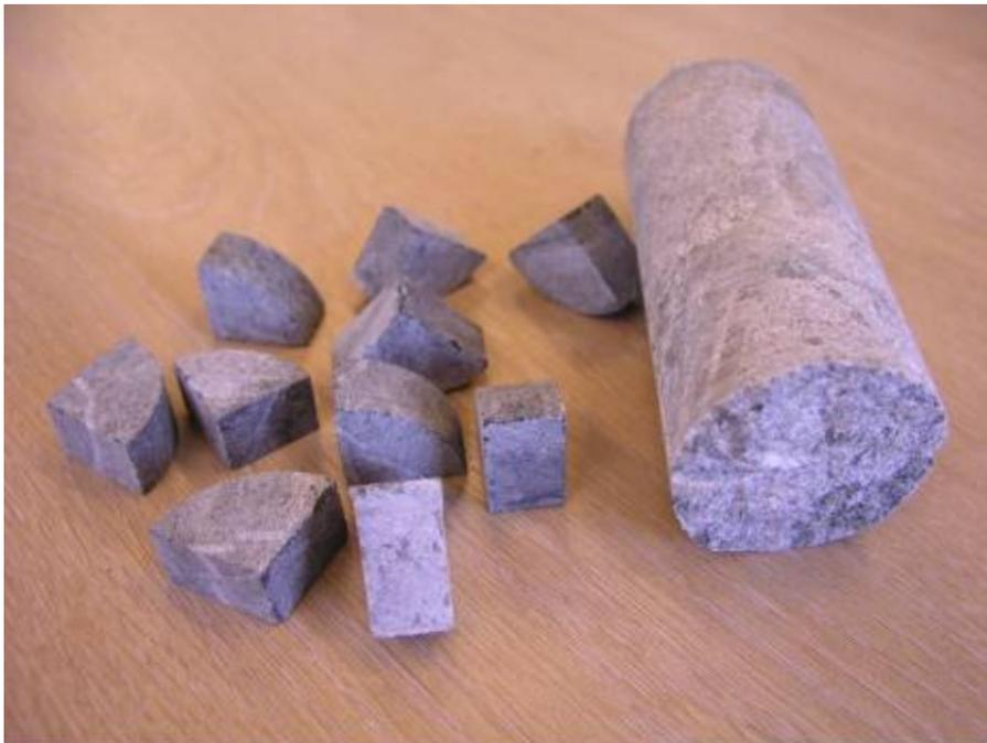
Figure 9 Particles selected for SMC testing from cutting drill core
