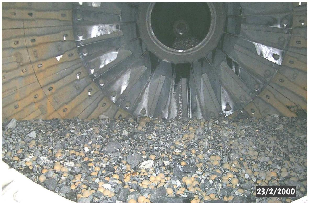
Figure 6 – Crash Stop of SAG Mill
