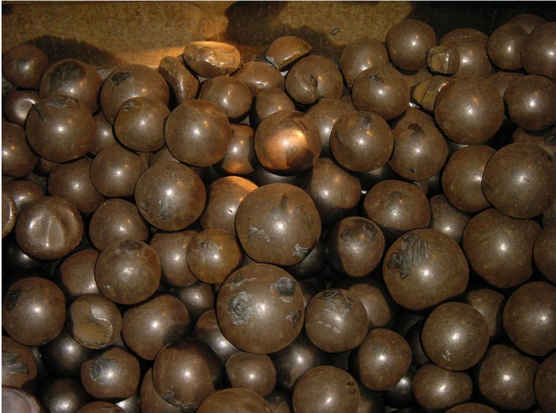
Figure 7 – Balls in a Mill After a Grind-out
