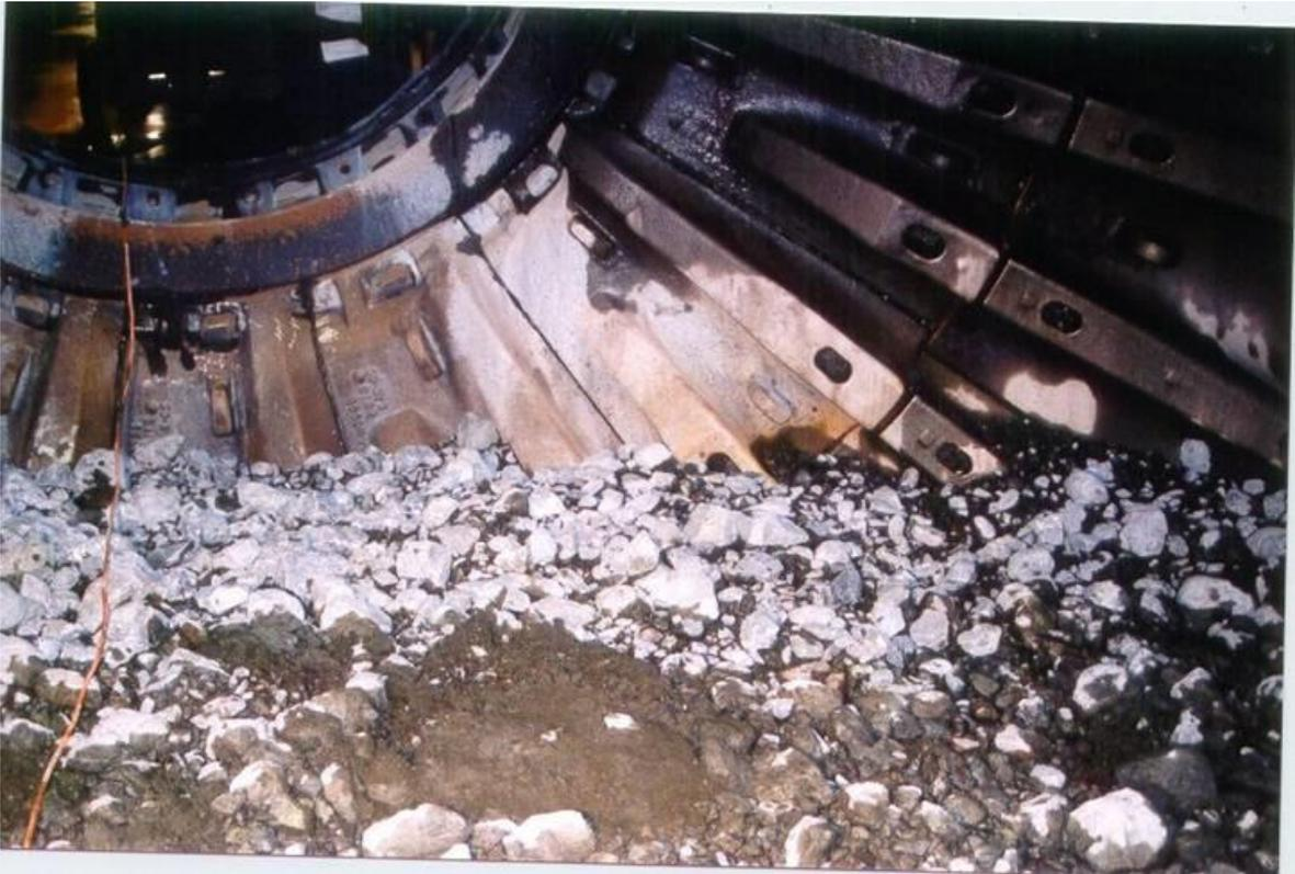
Figure 5 – Crash Stop of AG Mill
