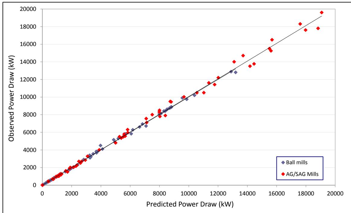
Figure 1 – Measured vs Predicted Motor Input Power
