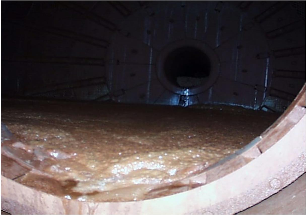
Figure 8 – View of the Inside of a SAG Mill with a Slurry Pool Problem
