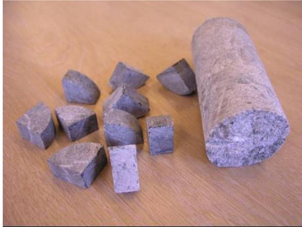
Figure A1 – Pieces Cut from a Drill Core Using a Diamond Saw
