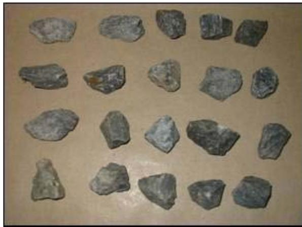
Figure A2 – Pieces Obtained by Crushing Drill Core
