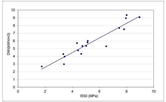
Figure 15 – Example of Correlation Between Point Load Index (IS50) and DWi
