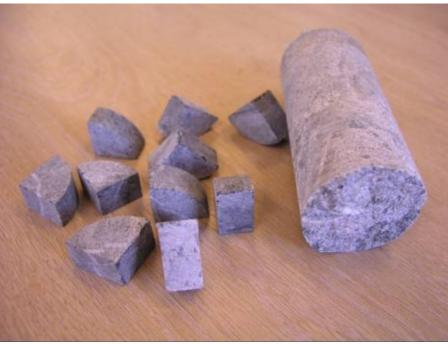
Figure 9 Particles selected for SMC testing from cutting drill core
