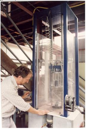
Figure 6 – Original JK Drop-weight Tester
