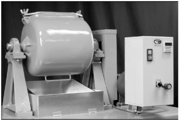
Figure 4 - Bond ball mill (after SME, 2019)
