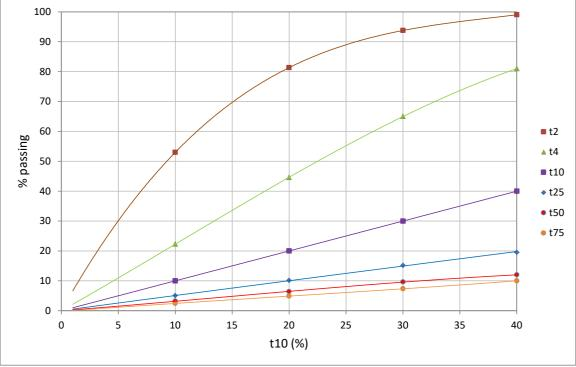
Figure 8 – Relationship Between the  $t_{10}$  and the Progeny Size Distribution
