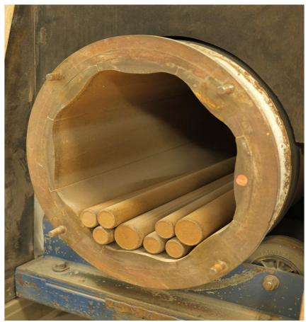
Figure 3 - Bond rod mill
