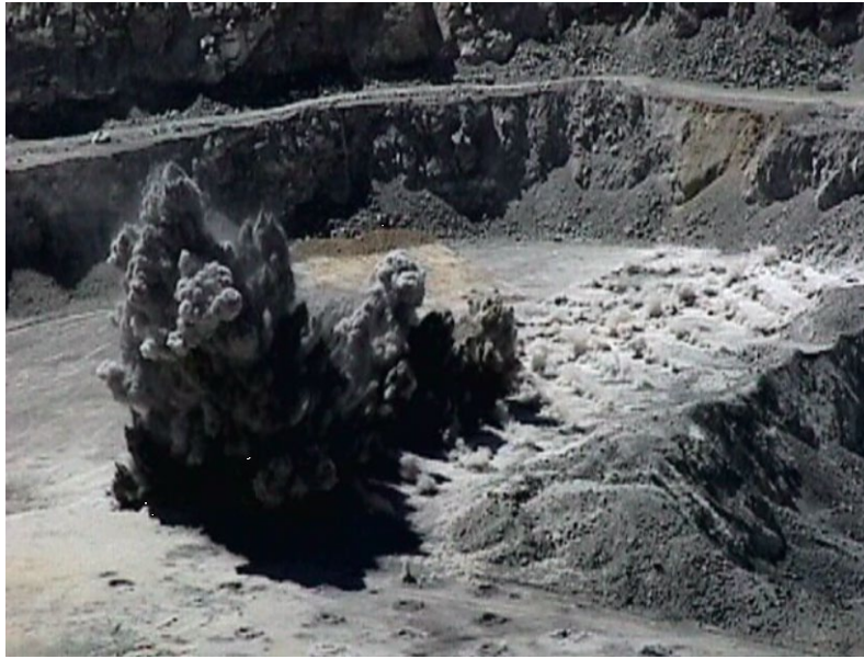
Figure 6 Cratering of Blasthole Collars
