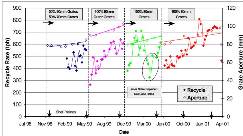
Figure 4: Pebble Recycle Load versus Grate Aperture and Liner Life
