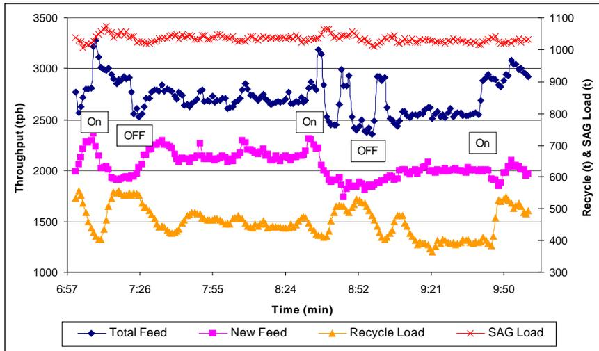
**Figure 8: Effect of Recycle Crusher on SAG Mill Circuit Stability**
