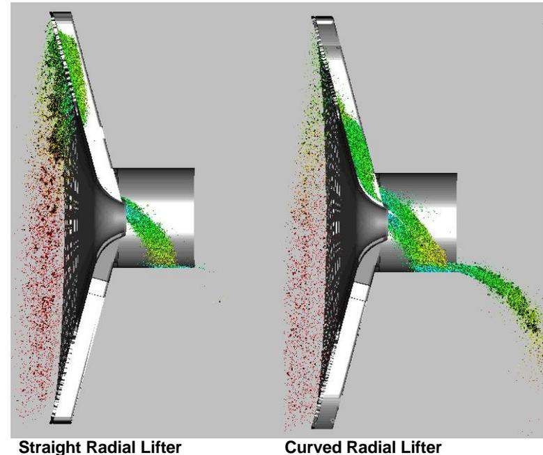
**Figure 7: Comparison of discharge rates from straight radial and curved pulp lifters.**
