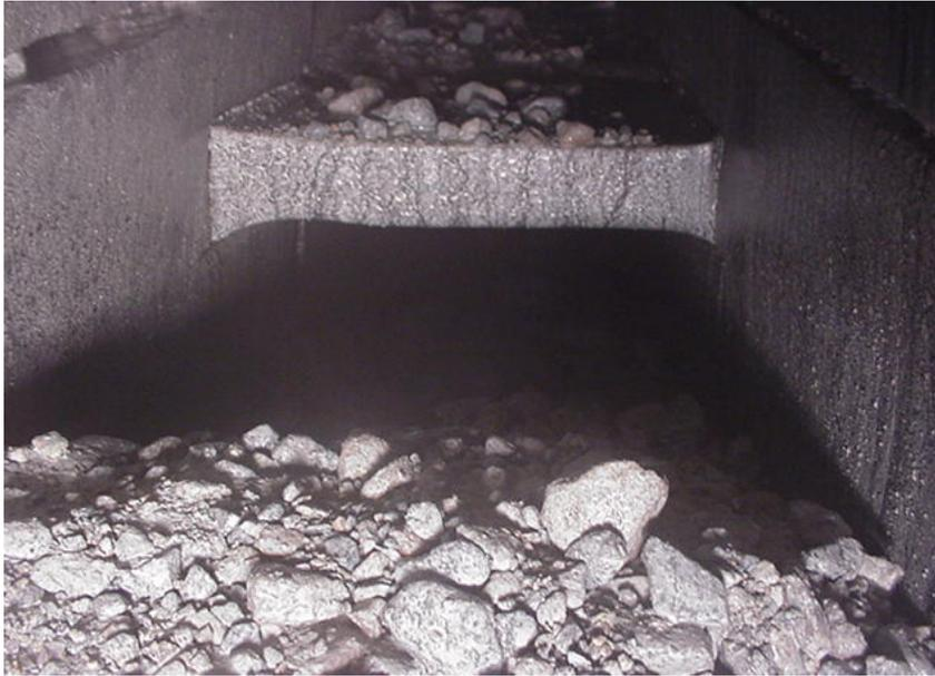
**Figure 6: Material Present on the Pulp Lifter Vane following a 'Crash' Stop**
