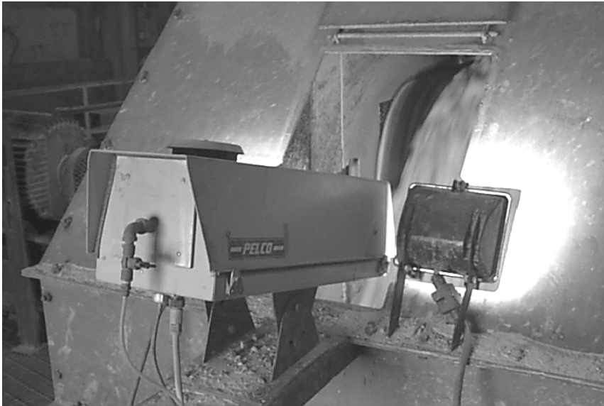
Figure 1: WipFrag Camera Installation
