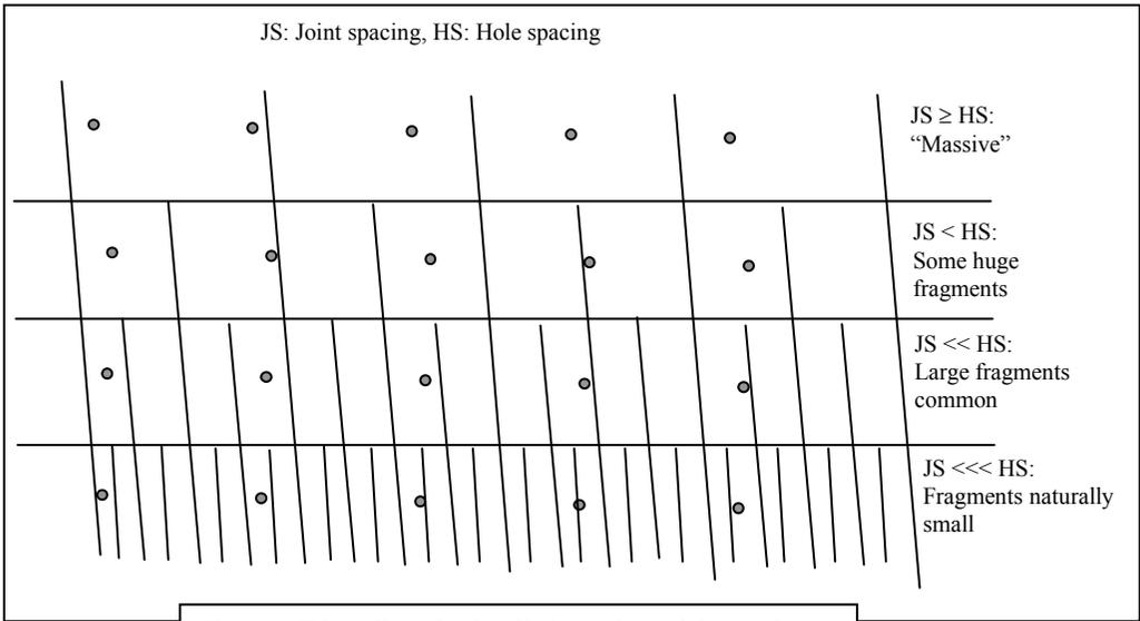
Figure 1. JPS – effect of ratio of hole spacing to joint spacing on blasting fragmentation.
