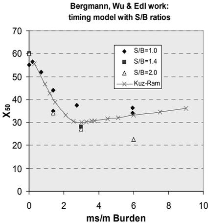
Figure 2. Tentative algorithm for the effect of inter-hole delay on mean fragmentation.
