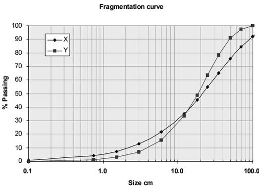
Figure 6. Effect of timing delay and precision on fragmentation. Identical geometry and powder factor, but  $Y$  has electronic delays with a 9 ms interval.  $X$  is pyrotechnics with a 25 ms interval.
