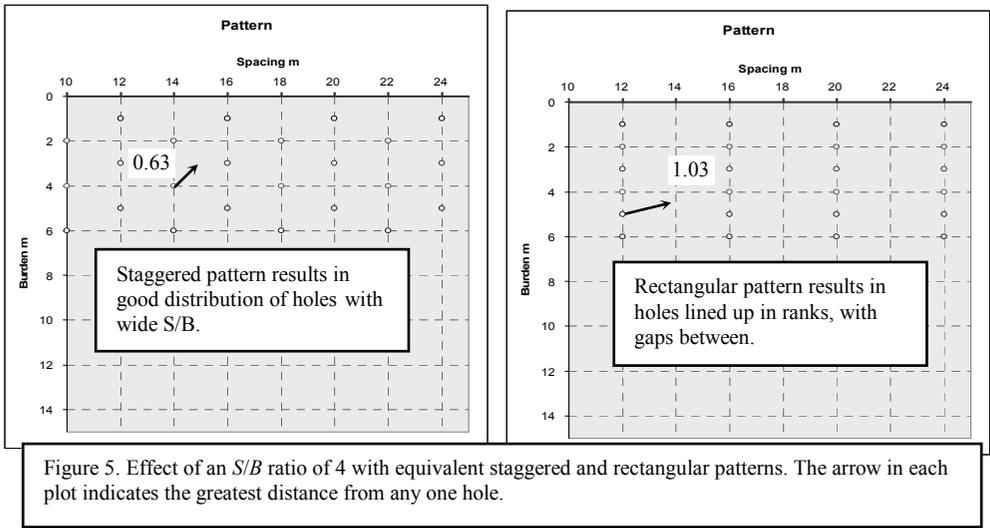
Figure 5. Effect of an  $S/B$  ratio of 4 with equivalent staggered and rectangular patterns. The arrow in each plot indicates the greatest distance from any one hole.
