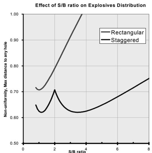
Figure 4. Effect of  $S/B$  ratio and layout on the maximum distance of any point from any hole.
