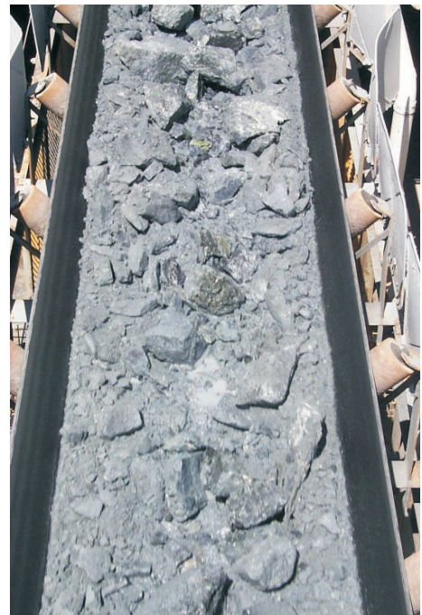
FIG 4 - View of muck on a conveyor.
