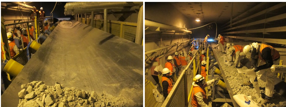
Figure 2 - Example of Belt Sampling - L1 (all material) on left and L2 (+ 75 mm) on right.
