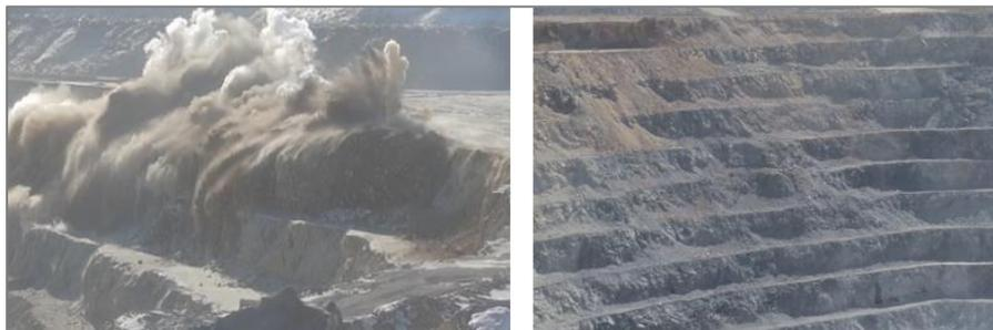
Figure 12 – Blast Movement into the Pit Void and Reduction in Catch Bench Capacity
