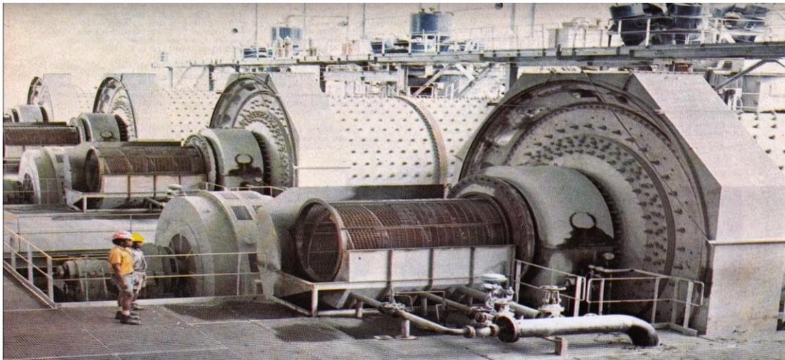
Figure 13 – Original Bougainville Ball Mills Refurbished and Sent to Pustynnoye, Kazakhstan
