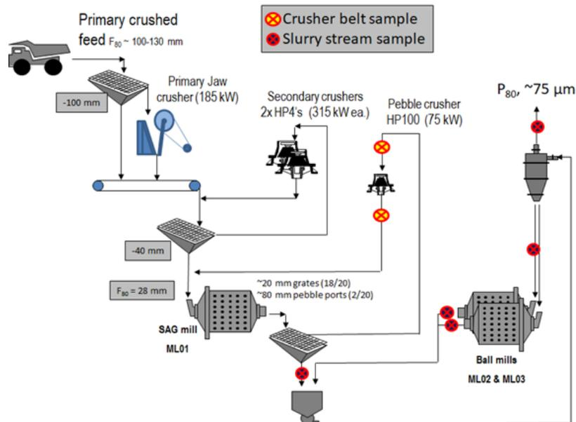
Figure 16 – Milling Circuit Survey Points
