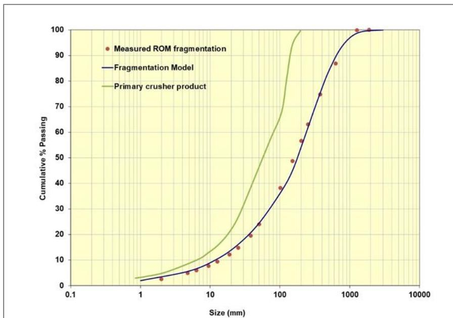
Figure 7 – Calibrated Fragmentation Model for the Base Case Blasts
