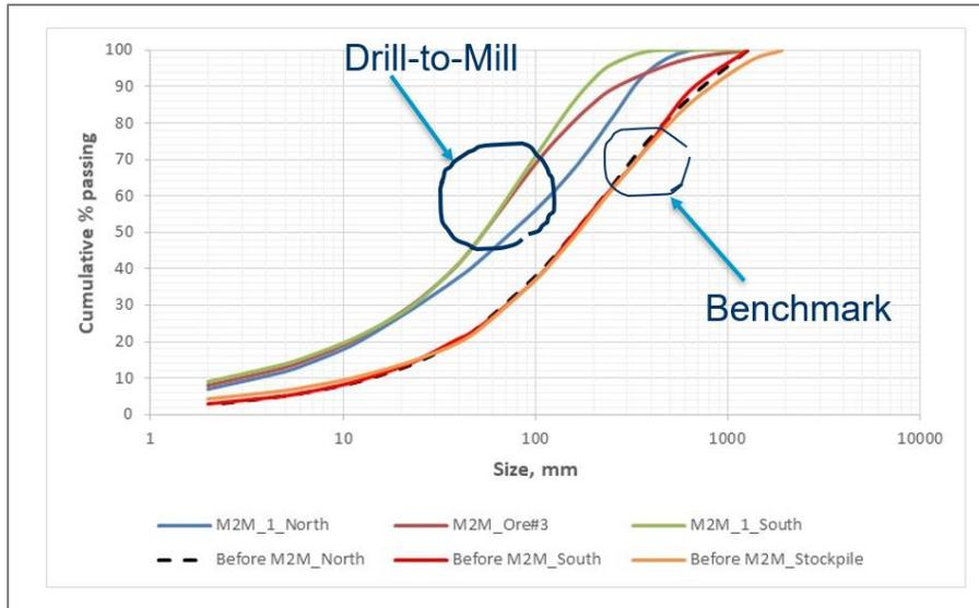
Figure 8 – Fragmentation Data from Benchmark and Drill-to-Mill Blasts
