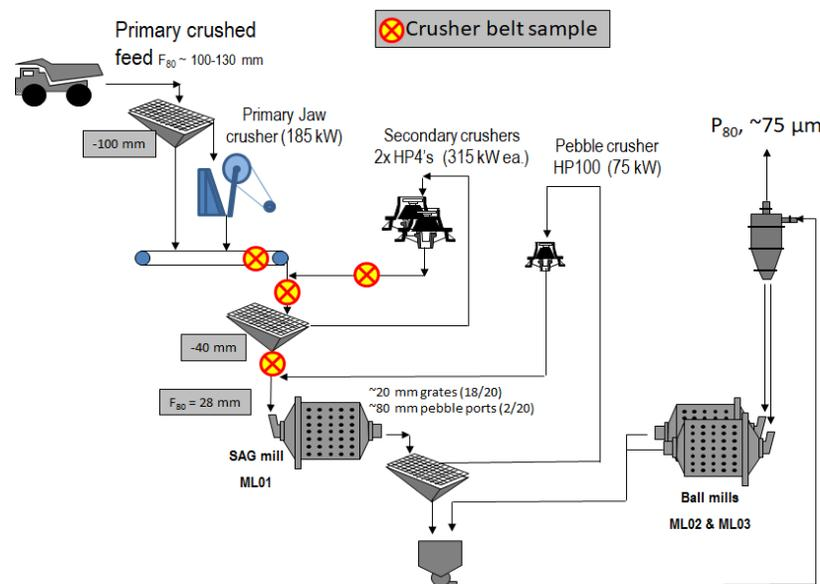
Figure 14 – Flowsheet Marking Points Where Crusher Survey Samples Were Taken
