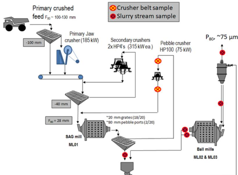
Figure 16 – Milling Circuit Survey Points
