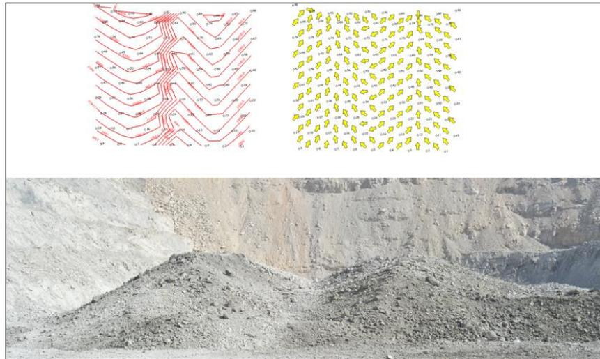
Figure 11 – Ore/Waste Segregation Blasting
