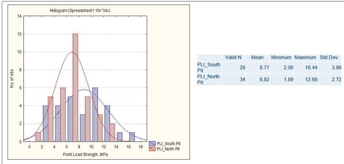
Figure 5 – Point Load Test Results for Lump Tests
