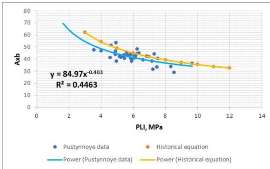
Figure 6 – Point Load Index, PLI vs. JK Drop Weight Test Parameter, Axb
