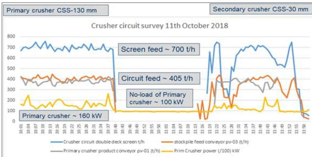
Figure 15 – Plant Information PI data from the crusher circuit survey October 11, 2018
