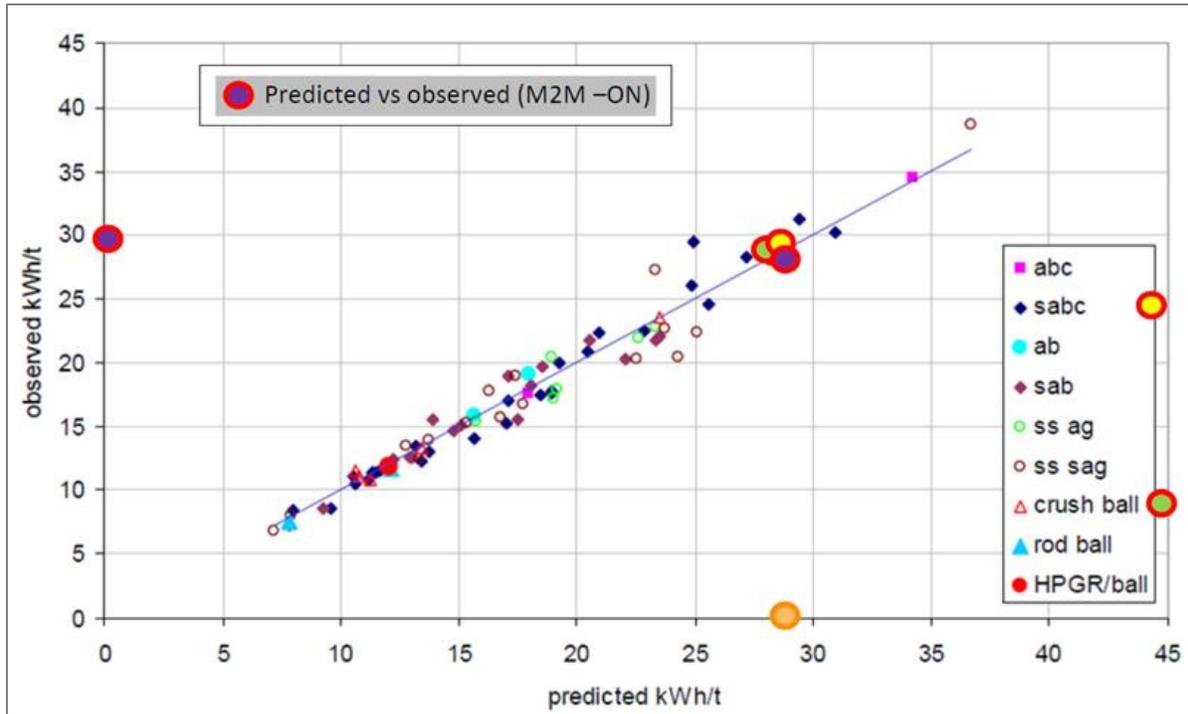
Figure 17 – Predicted vs. Observed Circuit Specific Energy for a 75 µm Target Grind Size
