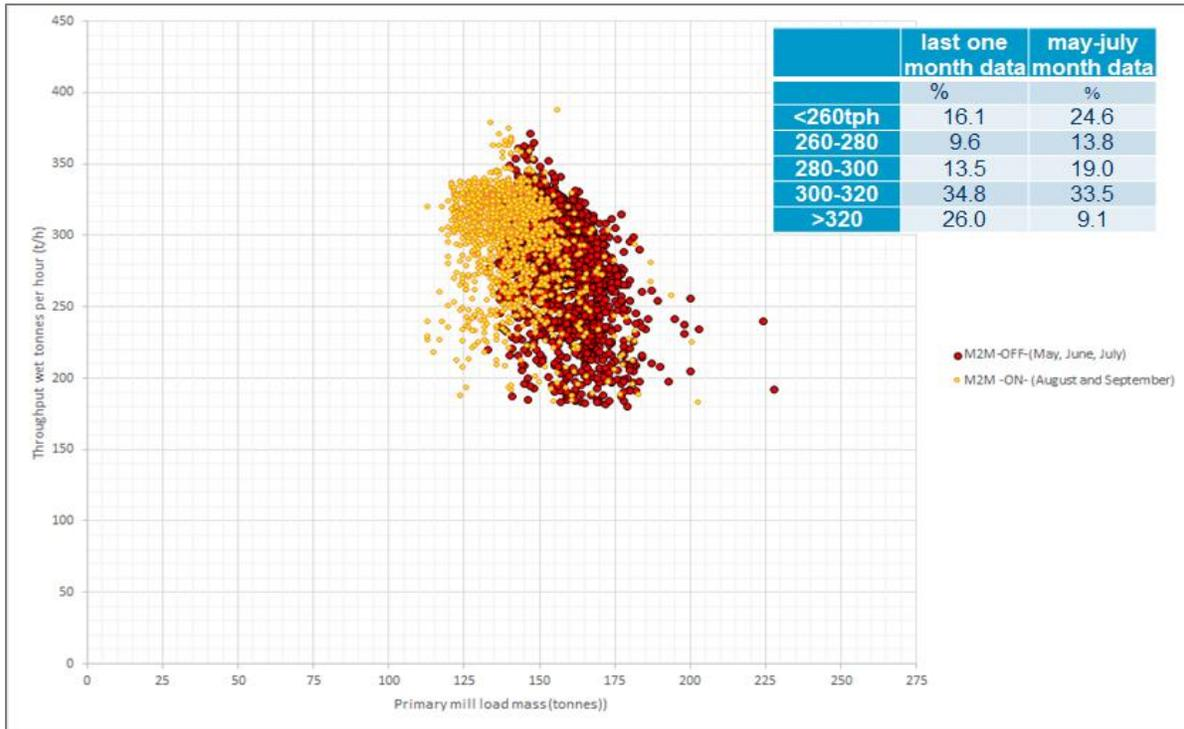
Figure 18 – SAG Mill Load (tonnes) against SAG Mill Throughput (t/h) – D2M ON/OFF
