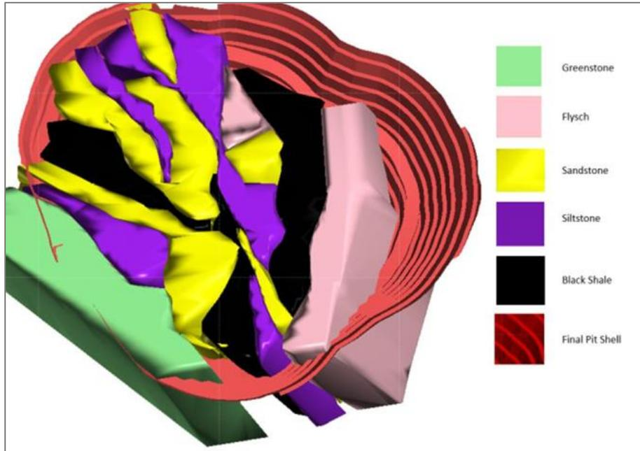
Figure 4 – Lithological Wireframes and Final Pit Shell View to the North (Brown & Marshall, 2017)
