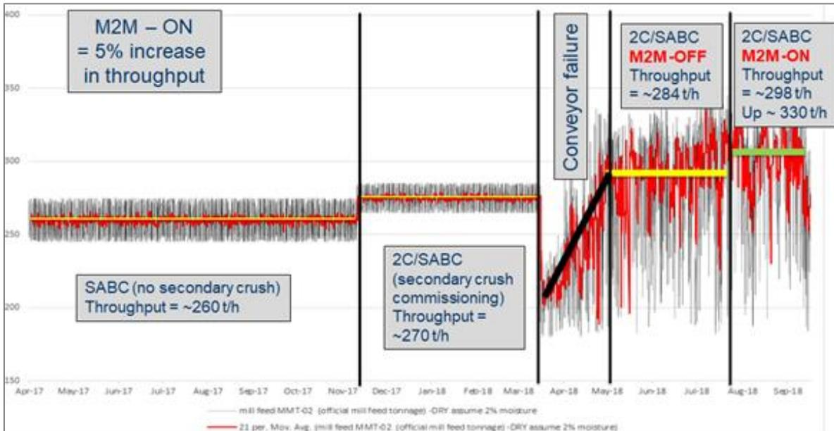
Figure 19 – D2M has Increased Throughput by ~5% to 298 t/h Since August 2018
