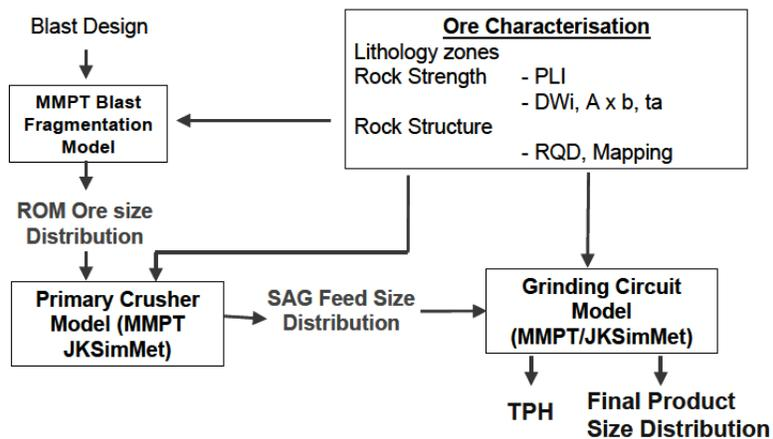
Figure 3 – Drill-to-Mill Methodology (Dance et al., 2006)
