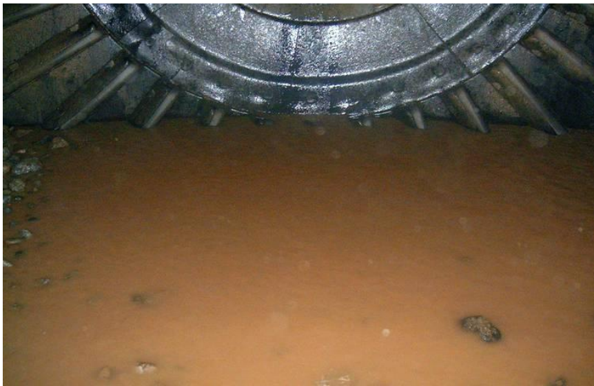
Figure 2 - Crash stop of SAG mill showing pooling
