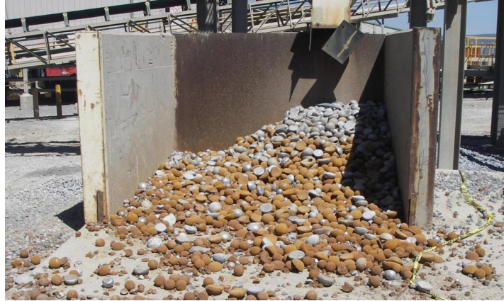
Figure 7 – North Mara SAG mill reject steel
